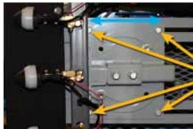
Loosen to slide rotating plate mounting plate
