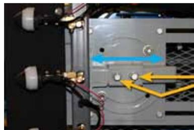
Loosen to slide sprayer arm out
